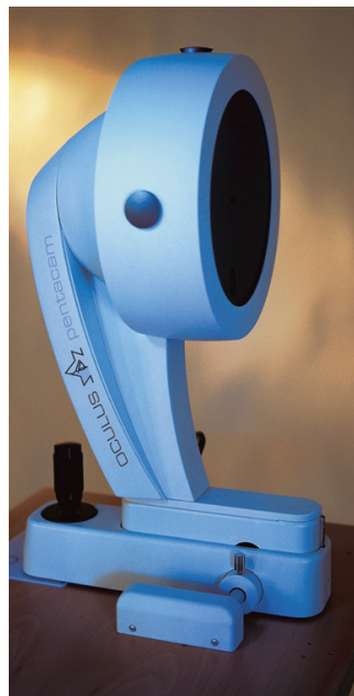
In addition to functioning as a topographer, pachymeter and camera, the Pentacam measures anterior chamber structures, displays corneal refractive power and provides densitometry data for monitoring cataract development.
